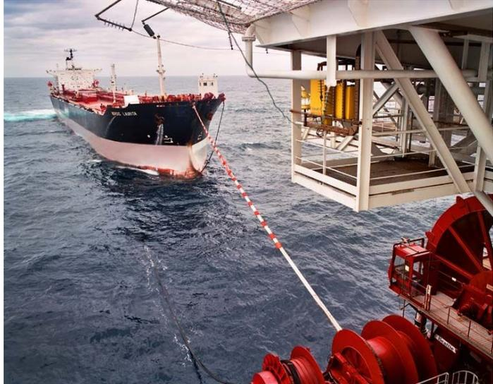
SPM do not constitute the weakest yield strength of MBL component of the entire system. Weak links, if fitted, should be designed, manufactured and tested under a certification scheme.
