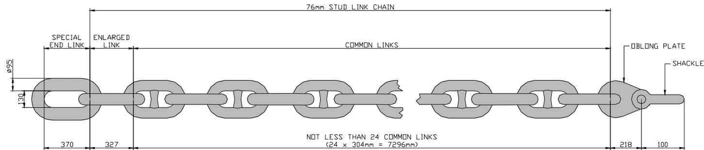
Chain manufactured, tested and inspected in accordance with IACS W22.
