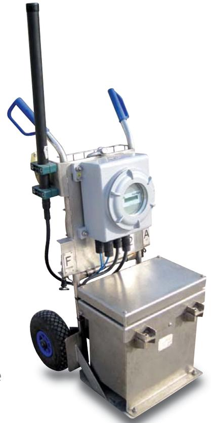
Until now, surge protection has either been monitored on board the single point moored (SPM) buoy, or even worse at the shore pumping station. By the time the Surge event is detected and the shore pump's stopped, it's often too late to prevent damage to subsea hoses and pipeline. The OILTECH Surge Protector (patent pending) offers a smarter and more sensitive way of detecting and automatically responding to pressure surges.
